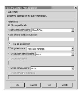
Reusable code will also be generated, when feasible, when you set **RTW system code** to Auto. Then, if only one instance of the subsystem exists, it will be inlined; otherwise a reusable function will be generated if other characteristics of the model allow this.
