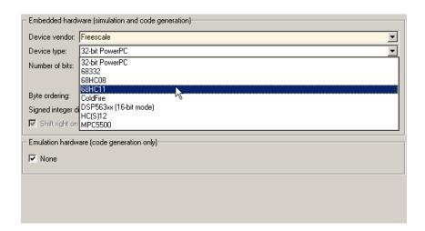
For more information about selecting code generation target hardware, see "Describing the Emulation and Embedded Targets" in the Real-Time Workshop documentation and "Device vendor" and "Device type" in the Simulink reference documentation.
