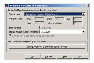
All but one of the parameters below the **Device type** menu are grayed out. This is because these characteristics have been preset for the default target (32-bit Generic), as well as for several dozen known target processors that you can select from that menu.
